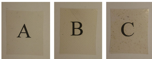
Figure 10. Photographs of films: (A) 1% CNW FD-P; (B) 2% CNW FD-P, and (C) 2% CNW FD. [Color figure can be viewed in the online issue, which is available at wileyonlinelibrary.com .]
